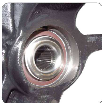
Picture 7: Clean off excess grease
