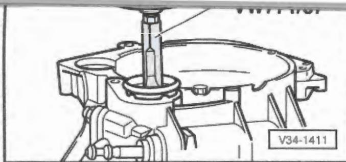
**Driving in flange shaft oil seal (drive in onto stop)**
